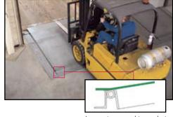
Innovative rear hinge design that creates a smooth transition between the leveller and the warehouse floor.
