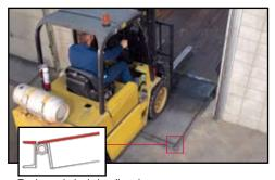
Traditional dock levellers have a gap at the rear hinge that creates a significant bump for fork-lift operators.
