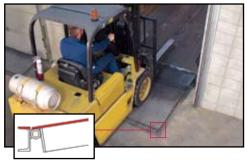
Traditional dock levellers have a gap at the rear hinge that creates a significant bump for fork-lift operators.
