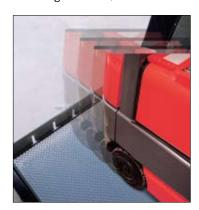
The barrier is automatically positioned when returned to the stored position after completion of the loading operation.
